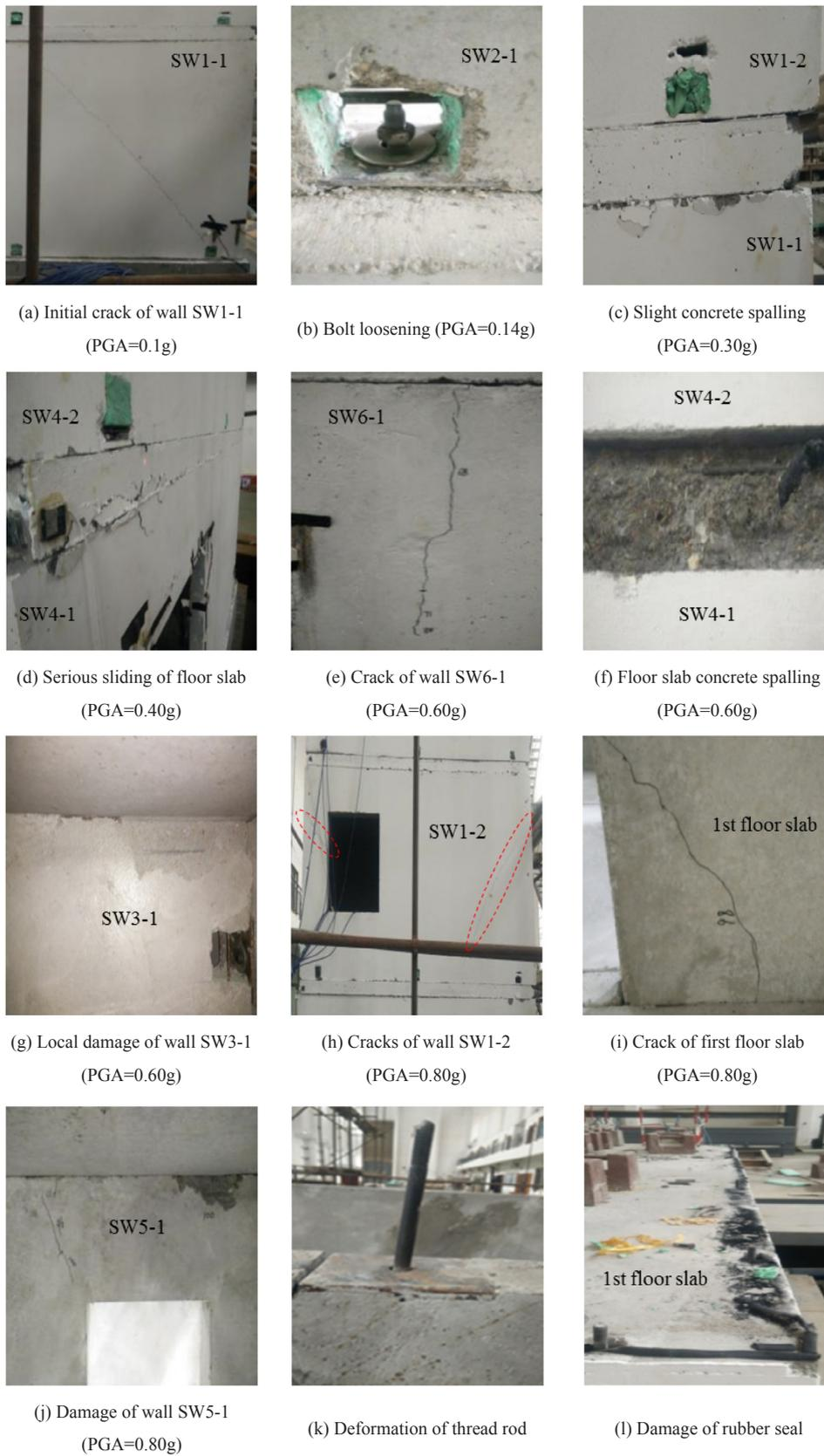
Fig. 9. Damage observations of the test model.
